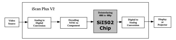
Figure 4: System Block Diagram
